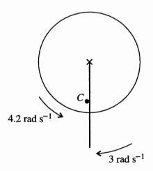
A disc is rotating about the same axis. The moment of inertia of the disc about the axis is  $0.56 \,\mathrm{kg}\,\mathrm{m}^2$ . When the rod is vertical, the disc has angular speed  $4.2 \,\mathrm{rad}\,\mathrm{s}^{-1}$  in the opposite direction to that of the rod (see diagram). At this instant the rod hits a magnetic catch C on the disc and becomes attached to the disc.
