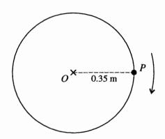
A wheel consists of a uniform circular disc, with centre O, mass  $0.08 \, \text{kg}$  and radius  $0.35 \, \text{m}$ , with a particle P of mass  $0.24 \, \text{kg}$  attached to a point on the circumference. The wheel is rotating without resistance in a vertical plane about a fixed horizontal axis through O (see diagram).
